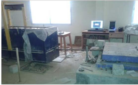
**Fig. 5: Shake table set up with laminar box**
